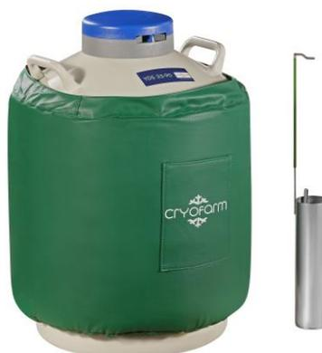
RÉSERVOIR POUR AZOTE LIQUIDE AVEC CAPACITÉ 35 LITRES ET COL 90 mm AVEC SIX CANISTERS À DOUBLE NIVEAU
